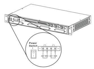
Figure 4-7 Front Panel AC Power Connection for NCT480
